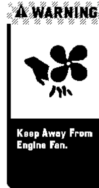
ENGINE FAN WARNING DECAL - LOCATED ON THE FAN SHROUD
